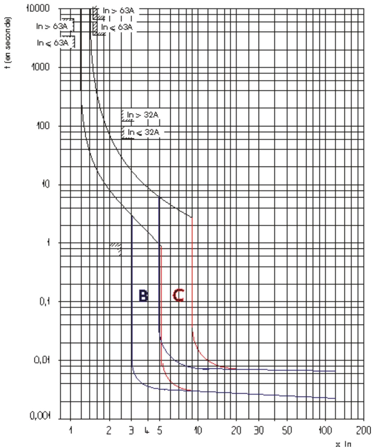
Thermal tripping at ambient temperature = 30°C
