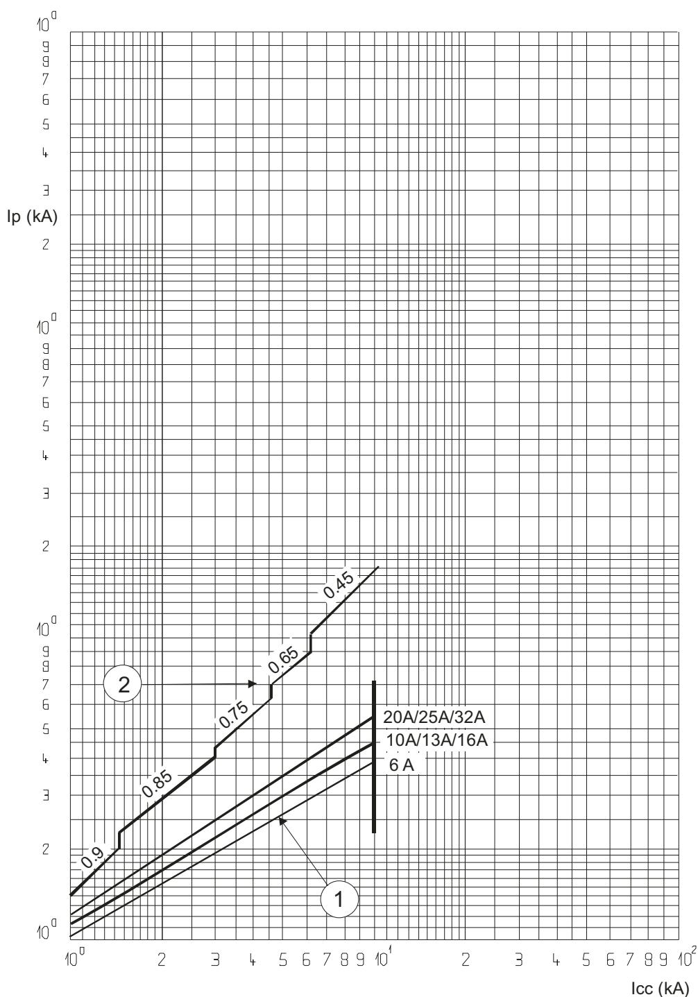
$I_{cc}$  = Symmetric expected short circuit current (effective value in kA) $I_p$  = Maximum Peak Value (in kA)
