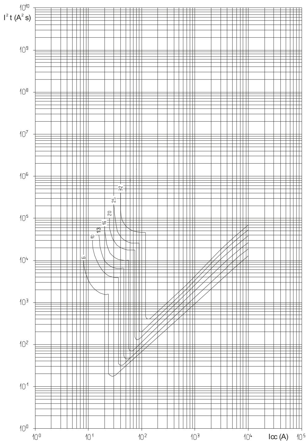
$I_{cc}$  = Expected short circuit symmetrical current (effective value in kA) $I^2t$  = Limited thermal stress (in  $A^2 s$ )
