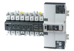
ATyS g M are modular automatic transfer switches with positive break indication. They are 2 or 4 pole (single or three-phase) devices. They have all the functions of the ATyS d M together with an integrated controller, giving them automatic features dedicated and mains/genset applications. They are intended for use in low voltage power supply systems where a brief interruption of the load supply is acceptable during transfer.
