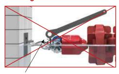
WARNING! When reel is under tension never hit thumb pawl with Ratchet Wrench to release catch lock. DO NOT allow reel spool to run free. This will damage teeth on spool and cause backlash of wire. It is also dangerous for the operator.
