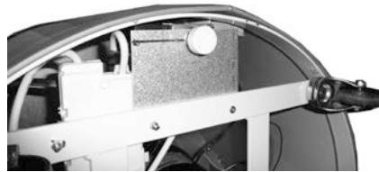
The thermostat is placed under the cabinet.
