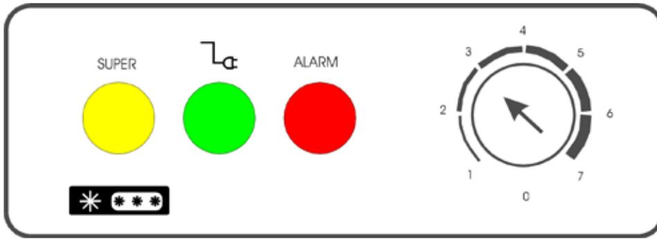
The thermostat can be adjusted on a scale from 1-7, which equals -15 to -25°C
