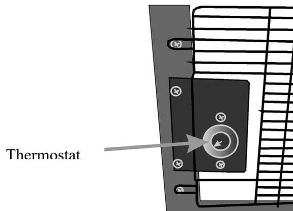
The thermostat can be adjusted with a scale of 1-6, which is equivalent to approximately 1-10°C
