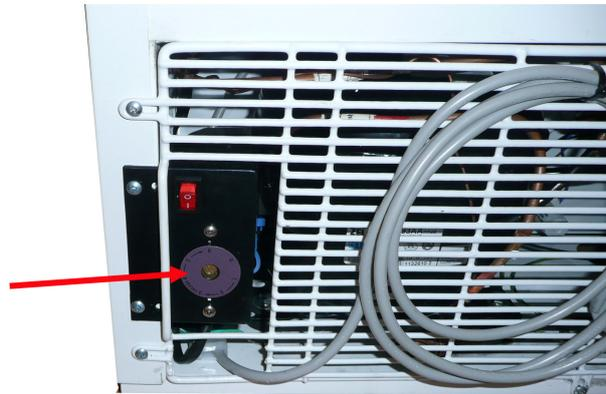
The temperature can be adjusted by using the thermostat button at the back of the cabinet. Set to position 5 on the thermostat scale. Place a thermometer approx. 10 cm inside the cabinet on the top shelf and check the temperature once it has achieved steady conditions. Turn the thermostat button clockwise if the temperature is too high or anti-clockwise if the temperature is too low.
