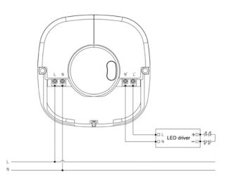
\*The sensor is designed for connect one load only. Connect more than one loads may damage the sensor.
