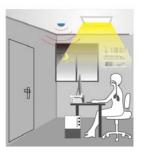
It keeps the light on even if the person is stationary for a long time, because it is maintained by breathing detection.
