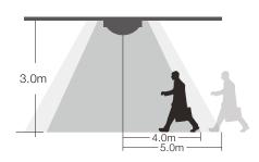
Movement Detecting Speed 0.3m/s
