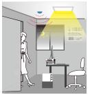
■When the ambient light is insufficient, a moving signal is detected and the light will turn on automatically.
