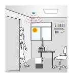
■ When the ambient light is sufficient, the light will not turn on even if the moving signal is detected.
