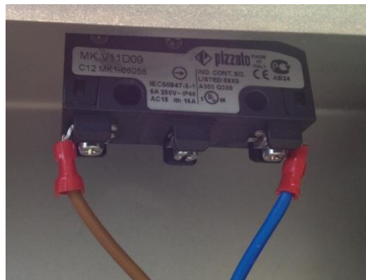
Figure 35. Lid switch wiring (new model)
