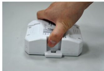
② The product has been correctly inserted into the panel lamp.
