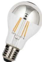
143611 LED FIL A60 TM Silver E27 DIM 8W (60W) 806lm 827
