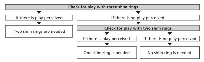
4. Install the necessary number of shim rings on to the axle, then install the freewheel body unit.
