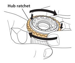
If the two hub ratchets do not engage, reset the position of the ratchets by turning clockwise while pulling up on the hub ratchet, then repeat the previous step. If the rings fail to firmly engage after several attempts, it may be indicative of a fault in the freehub body.
