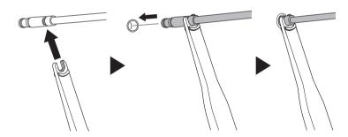
\* When disconnecting the EW-SD300, the method below can also be used. Lift the TL-EW300 straight up as indicated in (A), or use the TL-EW300 as a lever as indicated in (B).
