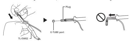
\* When disconnecting the EW-SD50, lift the TL-EW02 straight up as indicated in (A), or use the TL-EW02 as a lever as indicated in (B).
