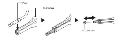
• When connecting the EW-SD300, the method below can also be used.
