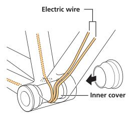
• If using a frame which does not have enough space between the inner wall of the bottom bracket shell and the inner cover to route the electric wires, use an inner cover which is sold separately.
