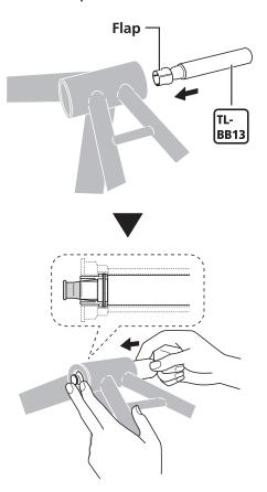
2. Tap the SHIMANO original tool with a soft face mallet to push out the adapter.
