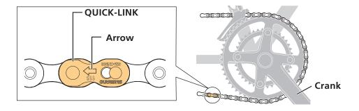
• When readjusting the length of the chain, be sure to insert the reinforced connecting pin from the same side that the chain cutter was inserted (the same direction as when the chain was cut).
