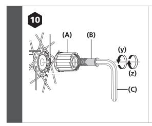
After removing the hub axle, remove the freewheel body fixing screw (inside the freewheel body), and then replace the freewheel body.
