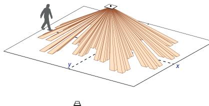
Detection pattern at floor level for 2.5 m mounting height
