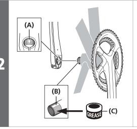
Set the wide groove area of the left crank arm into the axle of the right crank arm unit where the groove is wide.
