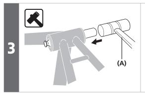
Tap the Shimano original tool with a plastic mallet until the end of the bottom bracket is ejected.
