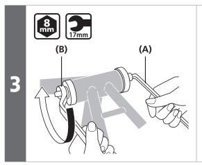
Press fit the bottom bracket by tightening with a spanner while making sure that the contact surface of the bottom bracket stays parallel to the contact surface of the bottom bracket shell.
