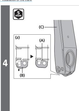
Push in the stopper plate and check that the plate pin is securely in place, and then tighten the bolt of the left crank arm.
