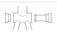
Use for a bottom bracket shell width of 86.5mm.
