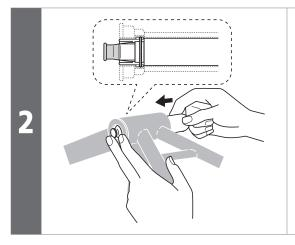
As shown in the illustration, hold down the flap with your fingers and push it in from the opposite side. (When pushed in, the flap opens.)
