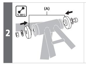
Insert the Shimano original tool into the bottom bracket.
