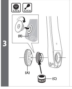
Use the Shimano original tool to tighten the cap.
