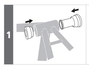
Insert the bottom bracket into the bottom bracket shell.
