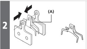
Set the pad fixing spring as shown in the illustration.
