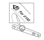
Temporarily attach the mount bracket to the frame.
