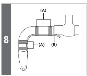
Temporarily secure the outer casing to the handlebar (by using tape or similar material).
