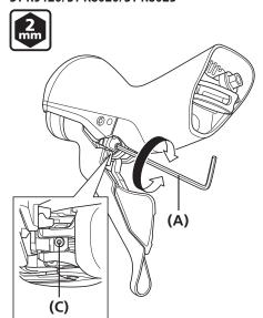
Turn the reach adjustment screw to position the lever unit.
