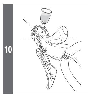
Once there are no more air bubbles in the oil in the funnel, change the angle of the handles so that bracket is 45°as shown in the illustration.
