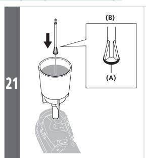
Plug the oil funnel with the oil stopper so that the O-ring mounted side is facing downward.
