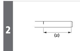
Put a mark on the brake hose beforehand as shown in the illustration so that you can check if the ends of the brake hose are secured to the hose mounts of the brake caliper and the dual control lever.
