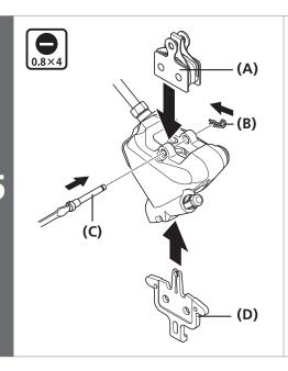
Install the new brake pads, the bolt, and the pad spacer (red).
