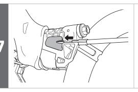
Finally, reinstall the cable cover.
