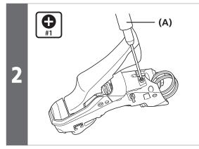
Remove the screw located at the bottom of the bracket, and then remove the unit cover
