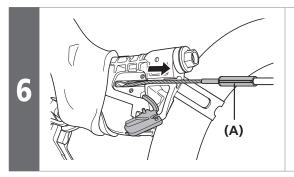
Put the inner cable through as shown in the illustration.
