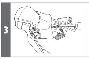
Use a pointed tool to pry out the SL cable guide.
