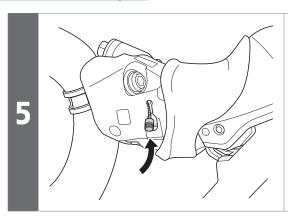
Insert the cable in such a manner that the inner end is housed in the unit.
