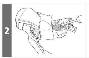
Remove the cable cover from the bracket using a screwdriver.
