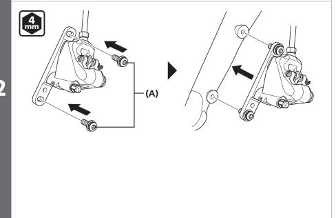
(A) Brake caliper mounting bolt A
