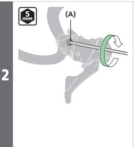
Use a 5 mm hexagon wrench to loosen the clamp bolt at the upper section of the bracket then tighten it after setting it on the handlebar. (A) Clamp bolt
