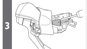
Remove the cable cover from the bracket using a screwdriver.
