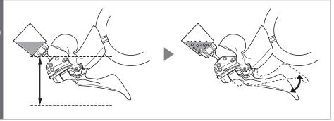
Make adjustments, such as changing the angle of the handlebar, so that the side of the bracket indicated in the illustration is 45° to the ground, and slowly apply and release the lever until no more air bubbles are emitted.
