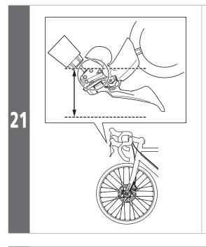
Make adjustments, such as changing the angle of the handlebar, so that the side of the bracket indicated in the illustration is parallel to the ground.
