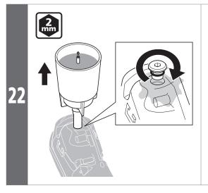
Remove the oil funnel and funnel adapter while still plugged with the oil stopper.
