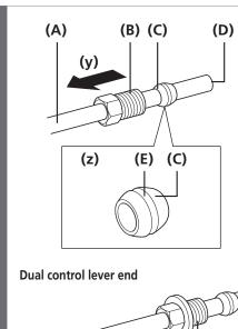
Pass the brake hose through the connecting bolt and olive, as shown in the illustration.
