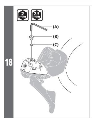
Remove the bleed screw and O-ring.
