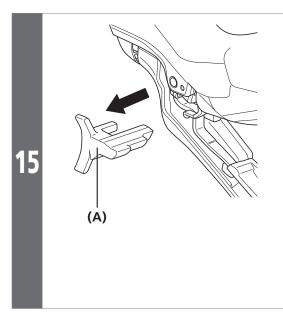
Remove the brake lever stopper.
