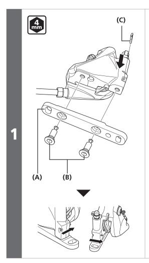
Attach the mount bracket to the brake caliper.
