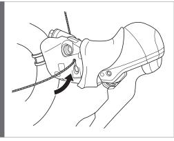
Put the inner cable through as shown in the illustration.
