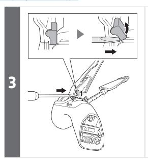
Rotate the main lever support in the direction of the arrow with a slotted screwdriver or an equivalent tool, and then remove the stopper.
