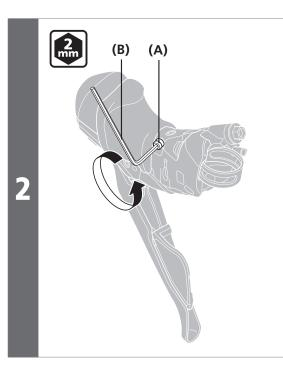
Turn the free stroke adjustment screw to adjust the stroke.
