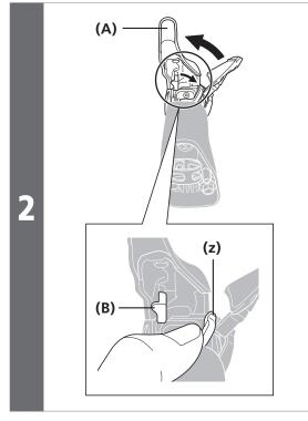
Hold the base of the main lever with the hands and then return only the main lever to the original position.
