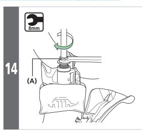
Tighten the flanged connecting bolt with an 8 mm spanner while pushing in the brake hose.
