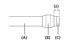
After checking that the olive is positioned as shown in the illustration, grease the screw threads of the connecting bolt.
