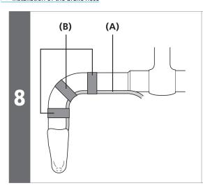
Temporarily secure the brake hose to the handlebar (by using tape or similar material).
