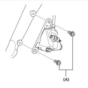
(A) Brake caliper mounting bolt A
