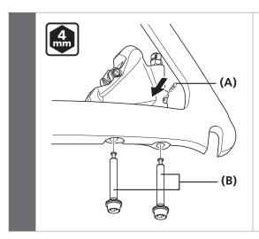
Attach the brake caliper to the frame.
