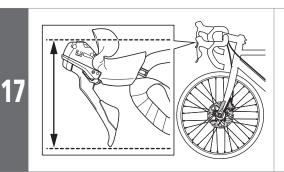
Adjust the position of the bleed screw so that its surface is parallel to the ground.
