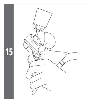
With the brake lever depressed, open and close the bleed nipple in rapid succession (for approximately 0.5 seconds each time) to release any air bubbles which may be in the brake calipers.
