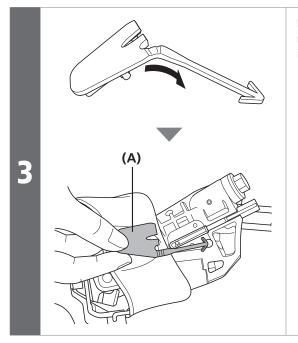
Before installing a new cable cover, make a slight crease on it and insert it into the hole in the bracket. (A) Cable cover
