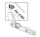
Insert the brake caliper mounting bolts A into the holes in the mount bracket first and then temporarily attach the mount bracket to the frame, as in the illustration.
