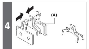
Install the pad fixing spring as shown in the illustration.
