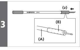
Insert the outer casing until it closely contacts with the end of the outer cap with tongue.
