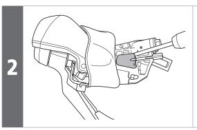
Remove the cable cover from the bracket using a screwdriver.
