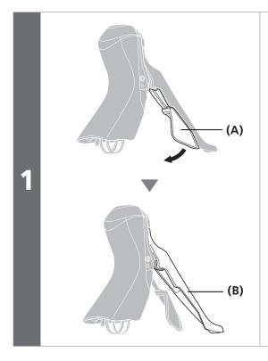
Operate the release lever 2 or more times, and then shift the main lever by 2 gears.
