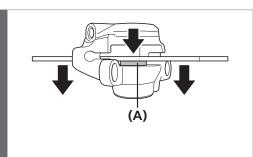
Use a flat-shaped tool to push the pistons straight back in as far as they will go, while being careful not to twist the pistons.
