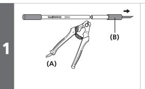
Use the cable cutter (TL-CT12) or an equivalent tool to cut the side opposite of the inscription.
