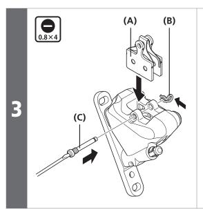
Install the new brake pads and bolts.
