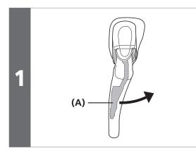
Operate the release lever 10 or more times and set the lever to the top position.
