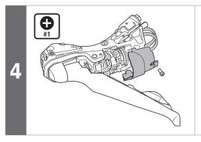
Reattach the unit cover and then tighten the screw.
