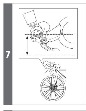
Make adjustments, such as changing the angle of the handlebar, so that the side of the bracket indicated in the illustration is parallel to the ground.
