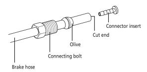
• Cut the brake hose so that the cut end is perpendicular to the length of the hose. If the brake hose is cut at an angle, fluid leaks may result.
