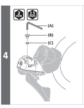
Remove the bleed screw and O-ring.
