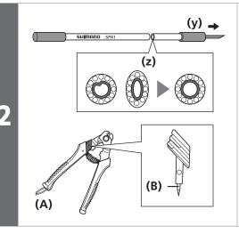
After cutting, expand the tip of the liner (Ø2.2 or more) with TL-CT12 or other narrow tool.
