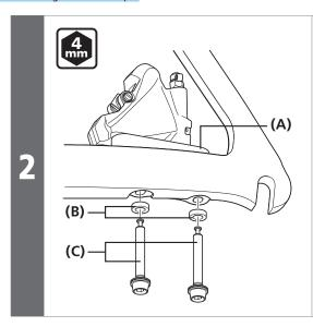
Use brake caliper fixing bolt C and a washer to secure the mount bracket to the frame.
