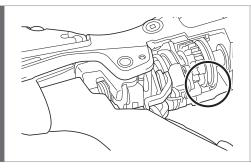
Pull out the inner end stayed on the cable hook of the winding body.
