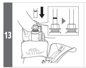
Insert the brake hose into the joint component until the mark on the hose is hidden.
