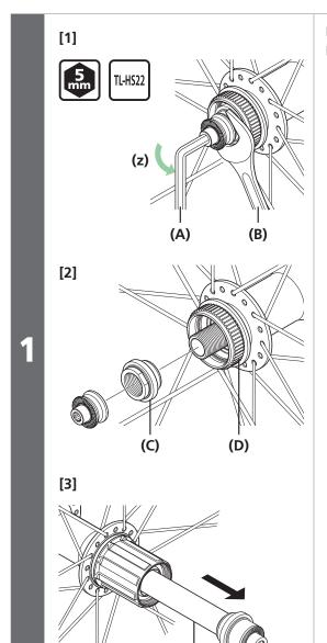
Pull out the hub axle by following procedures [1] to [3].
