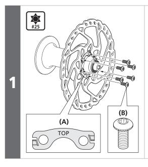
Install the disc brake rotor and rotor lock washers to the hub and tighten the holts
