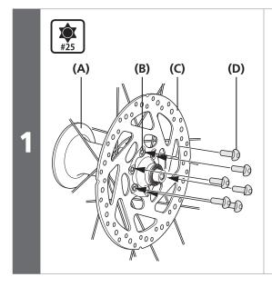
Install the disc brake rotor and the disc brake rotor tightening plate to the hub, and then install and tighten the bolts. **(A)** Hub
