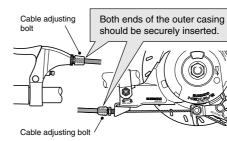
5. Push the cam transmission plate back until it stops. Then, while pulling the inner cable to apply the full amount of tension to the cable, tighten the inner cable fixing nut.
