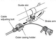
To install the brake cable again, carry out the above procedure in reverse
