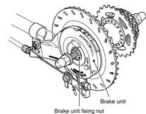
Tightening torque: 20 - 25 N·m {174 - 217 in. lbs.}
