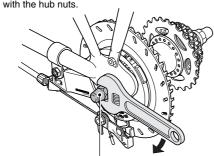
Hub nut Tightening torque: 30 – 45 N⋅m {260 – 390 in. lbs.}
