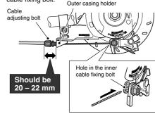
4. Check that both ends of the outer casing are securely inserted into the cable adjusting bolts of both the brake lever and brake arm.
