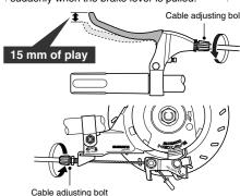
3. After depressing the brake lever to check the braking performance, secure the cable adjusting bolt with the cable adjusting nut.
