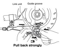
2. Slide the outer casing holder along the guide slot in the brake arm to remove it from the slot.
