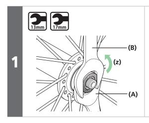
Use the spanner to loosen the lock nut on the double-lock section.
