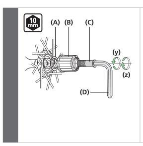
After removing the hub axle, remove the freewheel body fixing bolt (inside the freewheel body), and then replace the free-wheel body.
