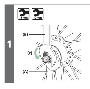
Use the spanner to loosen the lock nut on the double-lock section.
