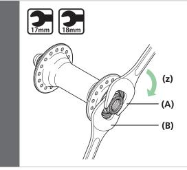
Install the hub axle, and then use hub spanners as in the illustration to tighten the lock nut so as to double-lock the mechanism.
