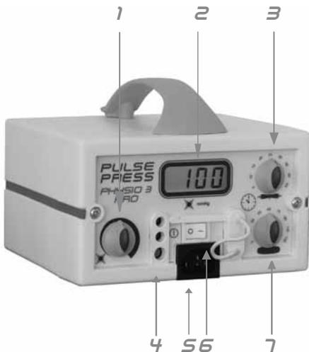
1. Pressure Control: This sets the air pressure in the garments. To set the pressure attach a garment and set the inflation to 120 secs. Switch the pump on and wait for the pressure meter reading to settle on a number. Now adjust the pressure, clockwise to increase, to the desired level, giving the system time to settle.
