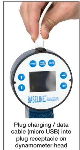
Plug charging / data cable (micro USB) into plug receptacle on dynamometer head
