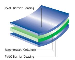
**500/600XS** Suitable for use as a single film for heavy duty packaging, tear-tapes, etc.
