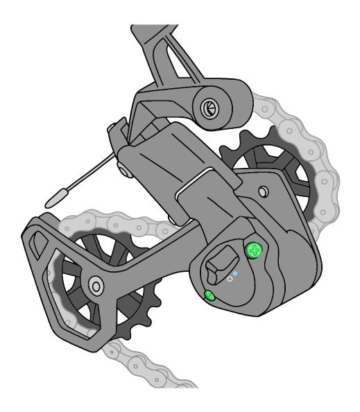
Use a T15 torx wrench to tighten the clutch assembly bolt a quarter turn at a time.
