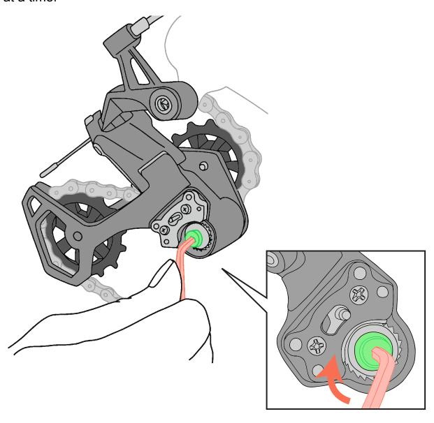
Push the derailleur cage forward after each adjustment to test clutch strength.
