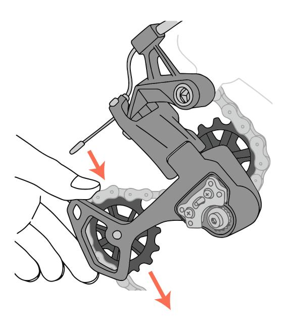
Replace the clutch cover and torque the screws to < 2nm.
