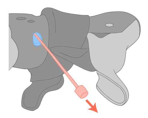
Rout the new cable through the cable port at the bottom of the shifter. Make sure the cable head is fully seated.
