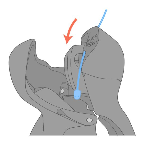
Route the new cable through the cable head seat and out through the barrel adjuster. Make sure the cable head is fully seated
