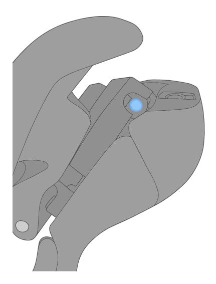
NOTE: Our MTB and IGH drop bar shifters do not have return springs. They rely on the derailleur's spring tension to up shift.
