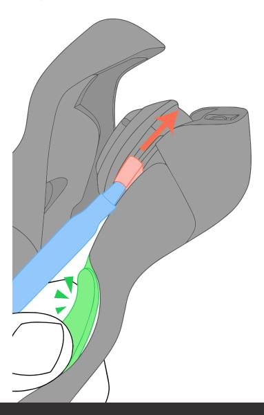
Press the thumb button until it stops clicking and the derailleur is in the small cog or small chainring position
